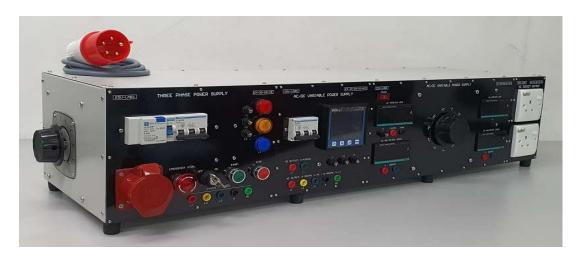
The system designed to provide all fixed and variable AC and DC supplies which necessary in an electrical machines laboratory to perform the experiment required and work project.
