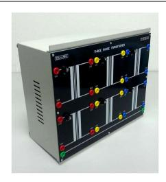
Each primary and secondary windings are divided in two sections to allow many possibilities of connection including star, delta and zig-zag.
