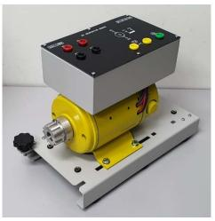
Nominal Power: 750W (1HP) Nominal Voltage: 220VDC Nominal Current: 2.0A 0 Nominal Speed: 1500 rpm 0 Terminals: 4mm Safety Socket Cooling Method: Self Cooling
