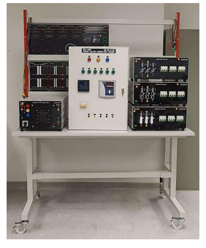
The unit is specially developed for use in electrical teaching laboratory for the purposed of demonstrating the basic concept and the operating principle of power factor correction system.
