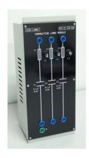
Configuration : STAR , DELTACapacitor : 0.1uF / 450V
