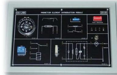
The EE-3500 Magnetism System Trainer is a comprehensive and self-contained system specially designed for Magnetism Circuit experiments training. The system consists of a Universal Lab Station and 5 Experiment Modules covering a wide variety of essential topics in the field of Magnetism Circuit. It is a time and cost-saving device for both students and researchers interested in developing and testing Magnetism Circuit's prototypes in institutions and universities.
