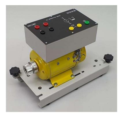
Load break direct current generator type for testing mechanical characteristics, convenience to measuring output torque & speed of motor on testing by attach a prime mover and torque sensor. To measures the variation of torque and speed by using AC/DC Generator Controller.
