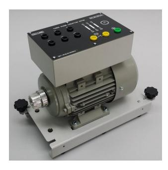
Single phase asynchronous induction motor, totally enclosed fan cooled
