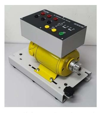
DC Motor / Generator Operation, suitable for series, shunt and compound excited connection
