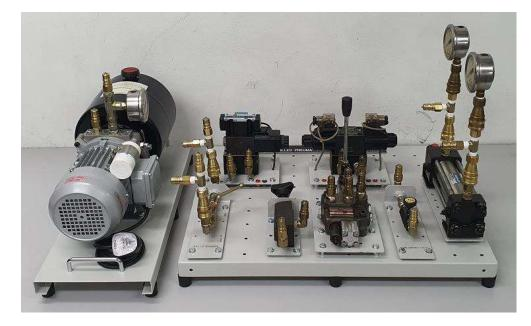
The Basic Electro-Hydraulics Trainers FH-202 is consists of actual industrial grade hydraulics components and parts which are commonly apply and used in industrial field. It is classified into basic level training experiments.
