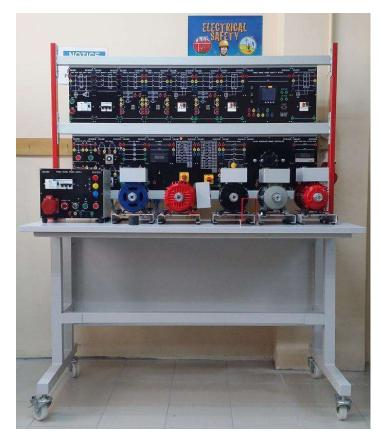
The EDU-LABS EM-68230 system consists of a series of modular slot-in panels modules housed in a compact epoxy coated casing. Each modules represents one or more electrical / electronic components or on block diagram of a complex circuits. All functional parts of the components are mounted inside the modules with circuit symbols/mimic diagrams screen printed on the front PCB panel and terminated at 4mm safety sockets for student experimental practice.
