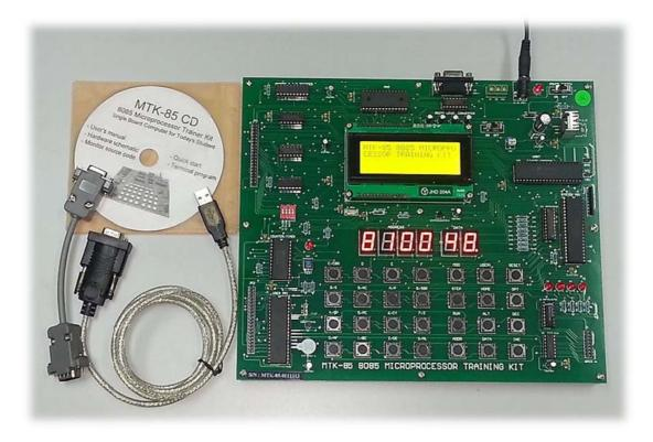
Single board computer built with a Intel 8085 Microprocessor, best for learning the fundamental of computer system.
