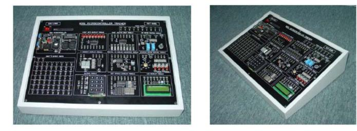
The 8051 microcontroller trainer is designed specifically for educational, institutes and individuals who are interested in 8051 microcontroller. It includes a Microcontroller Module with I/O ports Module, DC Power Supply Module and 9 standard application modules & 2 optional application modules. Come with complete software package for programming, source code editing, assembling, compiling, program writing.
