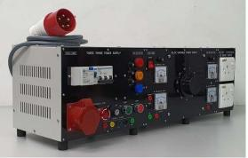
The system designed to provide all fixed and variable AC and DC supplies which necessary in an electrical machines laboratory to perform the experiment required and work project.
