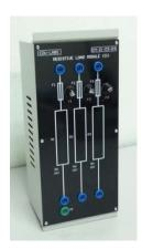
$\begin{array}{ccc} \circ & \text{Configuration} & : \text{STAR , DELTA} \\ \circ & \text{Resistor} & : 3x1.0 \text{ Ohm/5Watt} \end{array}$
