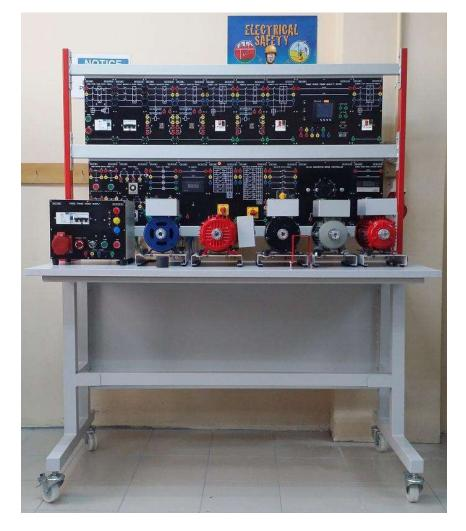
The EDU-LABS EM-68280Q system consists of a series of modular slot-in panels modules housed in a compact epoxy coated casing. Each modules represents one or more electrical / electronic components or on block diagram of a complex circuits. All functional parts of the components are mounted inside the modules with circuit symbols/mimic diagrams screen printed on the front PCB panel and terminated at 4mm safety sockets for student experimental practice.
