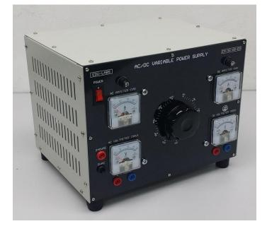
The system designed to provide all fixed and variable AC and DC supplies which necessary in an electrical machines laboratory to perform the experiment required and work project. The unit is contained in epoxy coated metal housing with clear front panel label and Output terminations by using 4mm safety sockets that make its easy and safety for student experiments.
