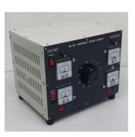
The system designed to provide all fixed AC and DC supplies which necessary in an electrical machines laboratory to perform the experiment required and work project.
